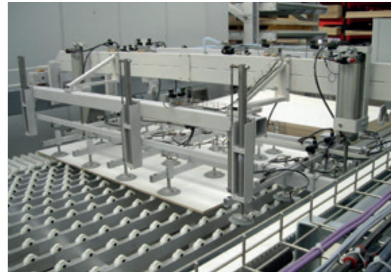
Vacuum in-feed: Transport of panels with sensitive surface
