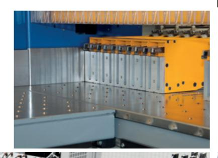
The aligning force on the cross aligning fence also enables heavy plates to be processed very precisely. Optional aligners in the roller table area ensure that even long strips are reliably pressed onto the aligning fence. This ensures maximum angular precision.
