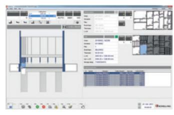
Display of the current cutting pattern, the cut, the order, and the material on the operator screen.
