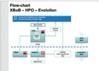
The operating data reporting of the MCS Evolution logs all relevant operating data, such as operating hours and the travel paths of the saw unit, feeder, pressure beam, etc. In addition, the running data of the
