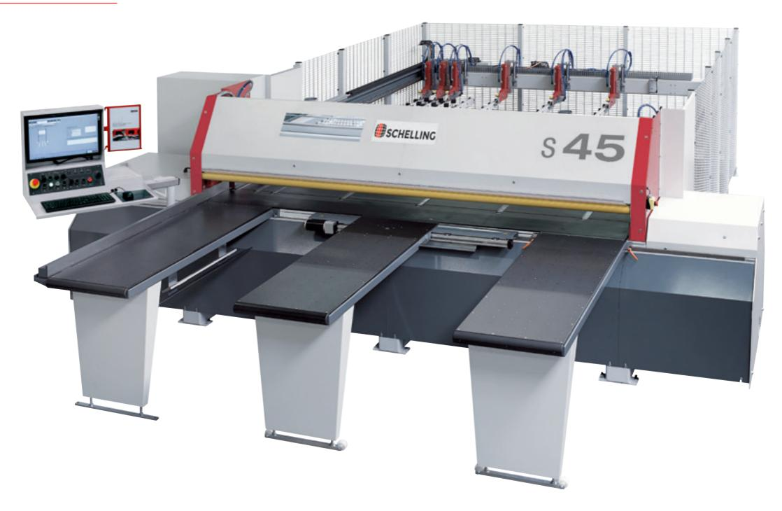
The Schelling s 45 opens up new potential where mitre cuts are required. This all-in-one machine combines the capabilities of two machines, thereby saving space, processing time and man hours. In addition, because there is no longer a need to change from one machine to the next, it provides more precision, more output, fewer errors, less damage and less waste.
